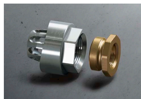
The press-in connection is suitable for steel pipes in accordance with DIN EN 10220/10255 and is available for steel pipe dimensions of 1½", 2", 2½", 3", 4", 5" and 6". It is equipped with a ¾" internal thread. A reducer for a ½" internal thread is also available.
