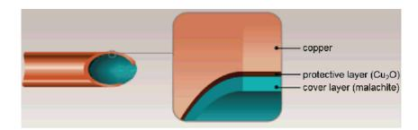
As a result of the greenish color, these desired coating layers are often confused with verdigris. However, verdigris is a salt of acetic acid i.e. a product of the reaction between copper and acetic acid. Since there is not generally any vinegar in potable water, the formation of any verdigris is impossible.
